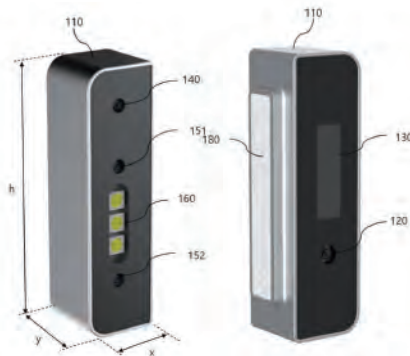
▲ A multi-camera device mounted on the side of the vehicle and a device that provides information on the situation of the vehicle environment
